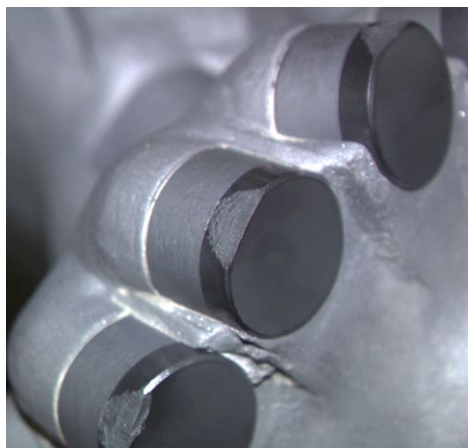
Fig. 8. Photo of field worn 1913 cutters with .160-in thick diamond and hoop interface geometry.
