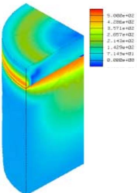
**Fig. 1. Maximum residual tensile stresses in a flat-interface 1313 PDC cutter.**
