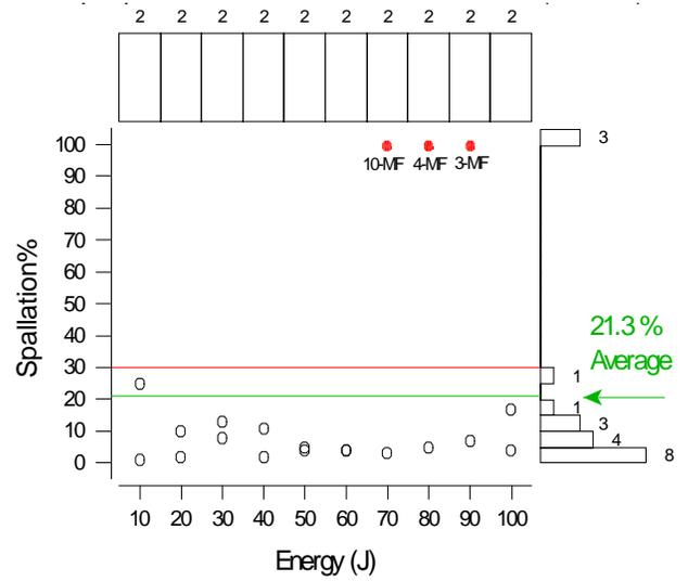
Fig 8. Drop-impact test results for a planar interface 1313 PDC cutter.
