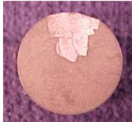
Fig 9. Typical example of general chipping or spalling cutter face damage.
