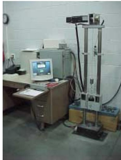
Fig. 5. Drop tower apparatus.
