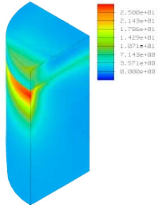
**Fig. 3. Strain energy distribution in a flat interface 1313 PDC cutter.**
