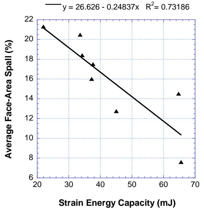
**Fig. 11. Strain energy capacity – drop-impact resistance correlation.**
