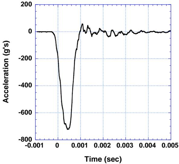
Fig. 7. Accelerometer response during a 100 J impact event.
