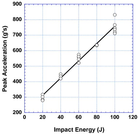
Fig. 6. Measured drop-tower acceleration as a function of impact energy level.
