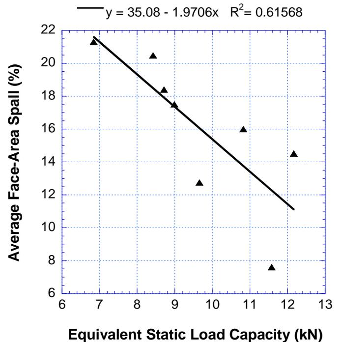
**Fig. 12. Equivalent static load capacity– drop impact resistance correlation.**
