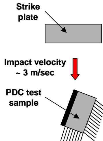
Fig. 4. Schematic of drop-impact test blow.
