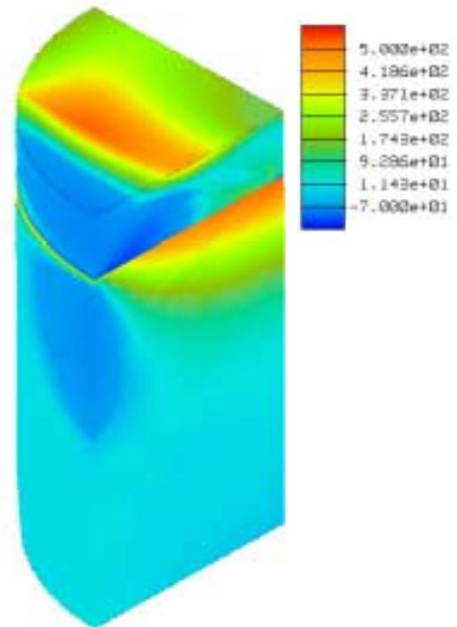
**Fig. 2. Maximum tensile stress due to the simulated drop-impact load combined with residual stress from Fig. 1.**
